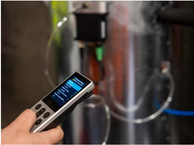
Indigo80 handheld device with GMP80P pump & tubing
