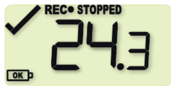
Figure 43: HAXO-16BT display with STOPPED visible while user is holding the START button
