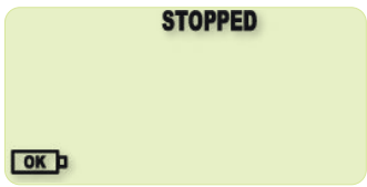
Figure 45: HAXO-16BT display after the START button has been released and has stopped recording
