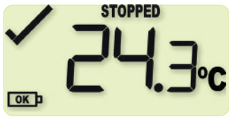
Figure 44: HAXO-16BT display while the user is pressing the START button, REC• disappeared
